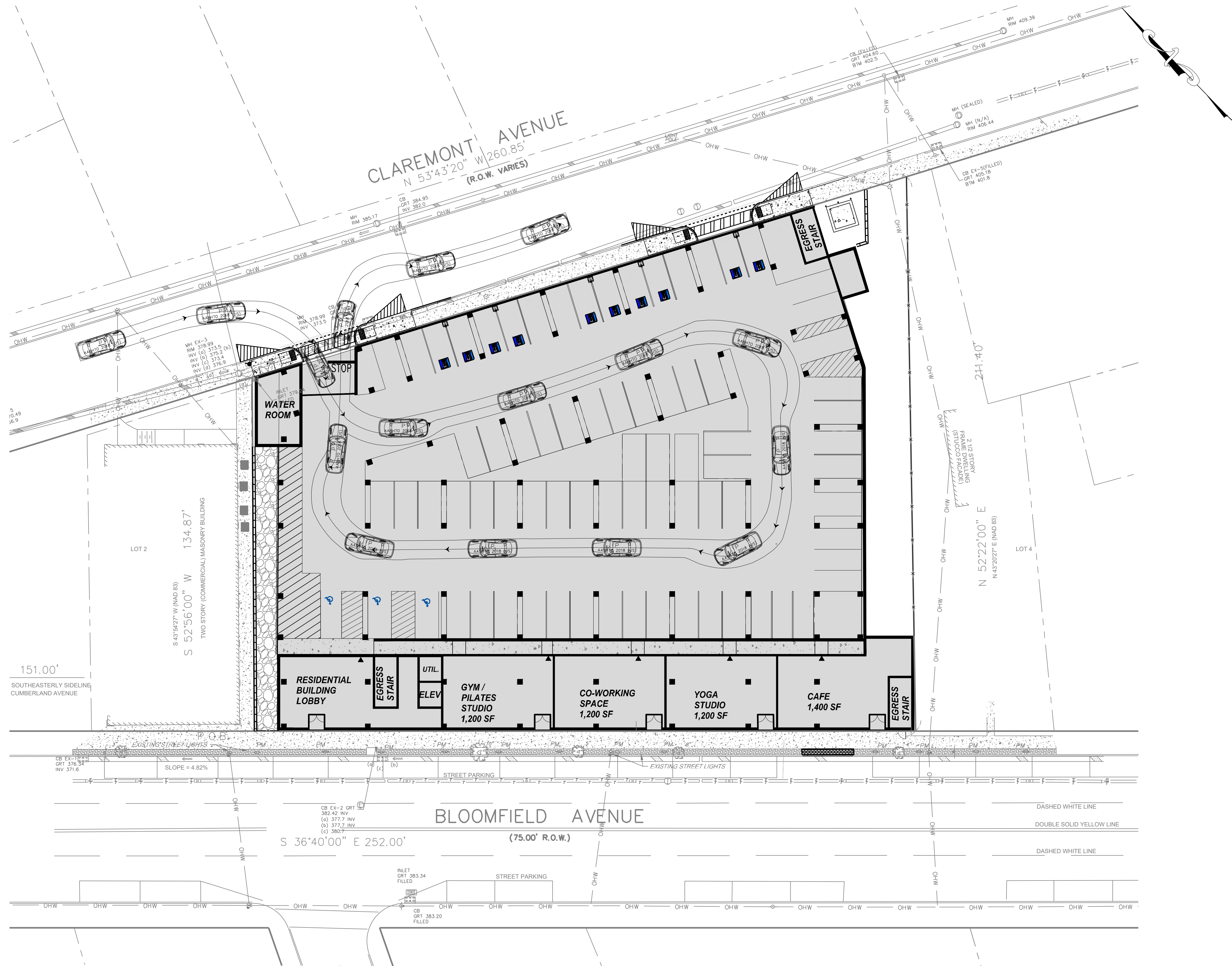
VEHICLE TURNING ANALYSIS LOWER LEVEL SCALE: 1" = 20'
