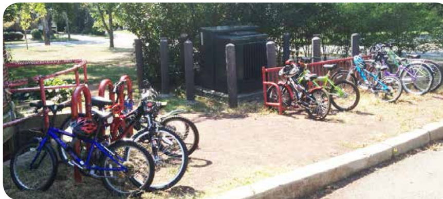
The ribbon rack on the left is preferred because unlike the comb rack on the right, it allows both the frame and wheels of the bike to be locked. Image: The RBA Group
