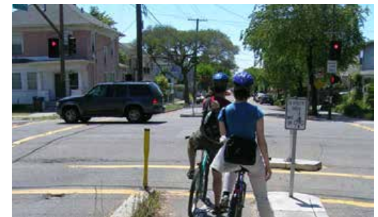
The signal at this crossing is actuated from an in-pavement loop detector. Image: NACTO
