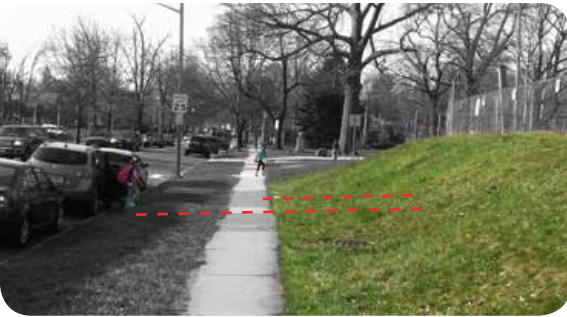
Poor example: The site lines of these two students from the sidewalk to the school yard are blocked by the height of the grassy slope. Image: The RBA Group
